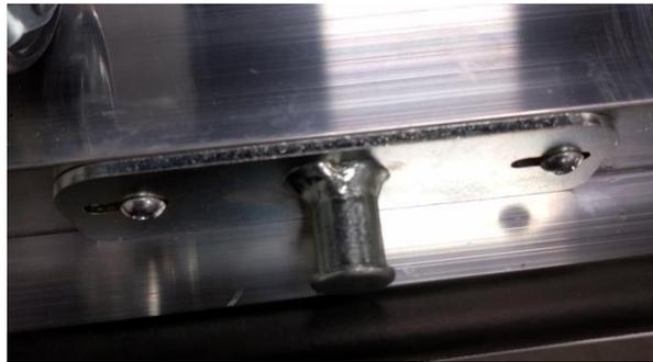
4. Make sure the latch is catching. Use your finger to close the latch and make sure it is holding latched in both positions. Also check to make sure the manual release lever at the latch is working. It is best to latch and unlatch these a couple times to make sure the manual release lever is not caught up in the latch.
